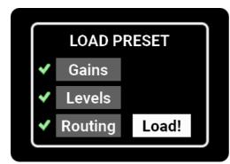
When loading a preset, you can also choose which parts of the selected preset should actually be loaded.
