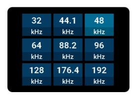
Pressing the MENU button again will bring you to the view in which you can select the internal sampling rate during INTERNAL operation.
