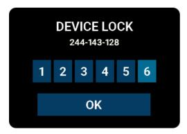
This function allows locking of the unit. When lock is active, only the headphone menu is accessible. Locking can only be done using the code provided on the sticker on the bottom of the device. The same code is also used for unlocking.
