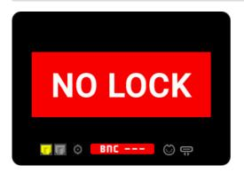
If no sampling frequency is detected at the selected clock source (ADAT or BNC), this error message appears.
