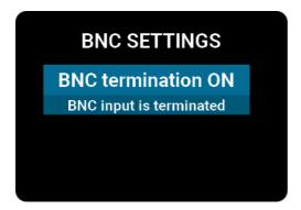
The BNC word clock input is internally terminated with a 75 0hm resistor. Termination should normally be turned on. For example, if you connect an output of another device with a BNC cable directly to that input.
