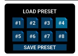
In the PRESET display you can save and load one of eight presets. For saving, use the knob to navigate to SAVE PRESET. Loading a preset is done simply by selecting one of the preset numbers.
