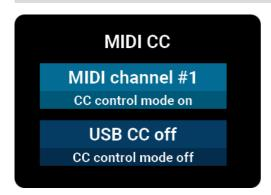
Here you can choose whether the device can be controlled via Control Messages. Select the desired channel, or "off" to deactivate. You can set this independently for the physical MIDI port (3.5mm jack on the back), or the USB connector. The table of CC commands can be found on our website. In addition to MIDI CC commands, the device can also be controlled remotely via the RemoteFish software.
