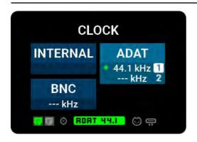
In the CLOCK display you can set the clock source and sample rate.
